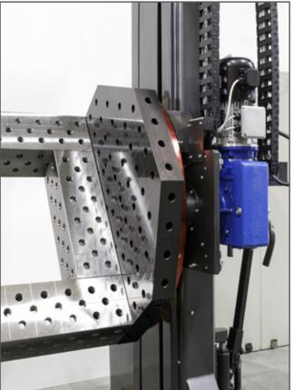
The use of octagonal tables and / or multi-hole bars gives the device great flexibility in the placement of the pieces.
