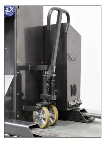
The movement of the two machines is particularly easy because of the manual lifting device, useful even when changing the sizes of the workpieces.
