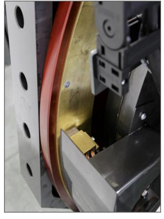
Both the columns are provided with ground bearing: carbon/graphite brushes are kept under pressure against a brass surface to prevent oxidation during inactivity.
